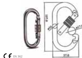
LX03 Carabiner/ Screw Gate Alloy Steel. MBL: 22kn
