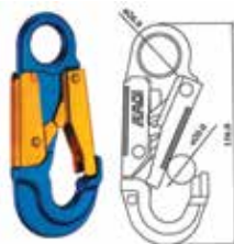
LX05 Snap Hook Aluminium Alloy MBL: 27kn
